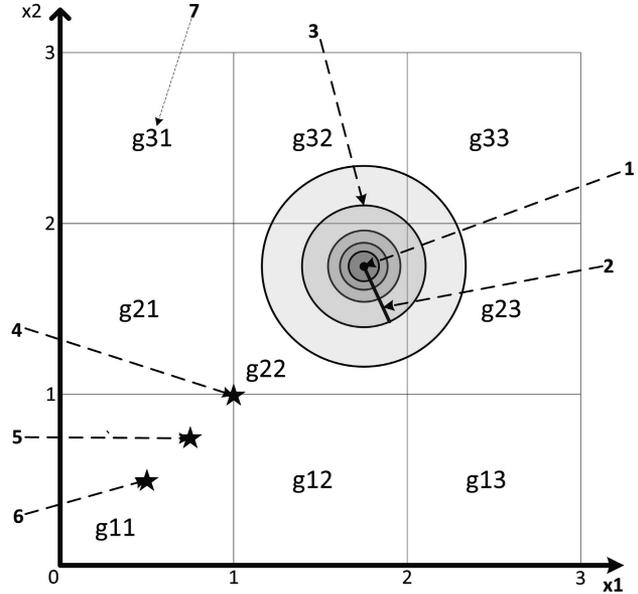
**Figure 1.** Projection range of picture  $G$ , 1 – center of the PLC projection  $\mathbf{x}_0$ , 2 – dispersion radius  $r$ , 3 – equipotential line of signal power, 4, 5, 6 – center location of the PLC projection  $\mathbf{x}_0$  relative to model receiver, 7 – subfield  $g$  of the sub range  $G$  equal to elementary photoreceiver.
