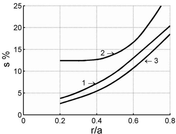
**Figure 5.** Dependence root-mean-square error of coordinate location on dispersion radius (SC).
